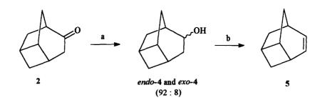
a) LiAlH4/diethyl ether b) HMPA, 230 °C In order to prepare 4 and 5, tricyclic ketone 2 was first reduced with LiAlH<sub>4</sub> to give 70% yield of 4 as a mixture of *endo-* and *exo-* stereoisomers (product ratio 92:8).<sup>7</sup> Subsequent dehydratation of 4 with HMPA at 230 °C afforded 5 as the sole product.<sup>8</sup>
